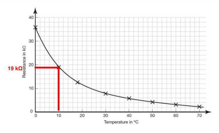
Use the x axis to work out the resistance at a specific temperature
